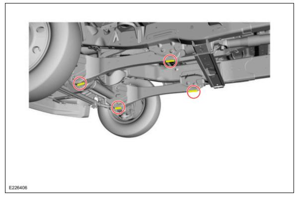
NOTICE: When raising a vehicle on a hoist, use care when positioning the hoist adapters prior to lifting the vehicle so that hoist arms do not interfere with the surrounding suspension or steering linkage components.
