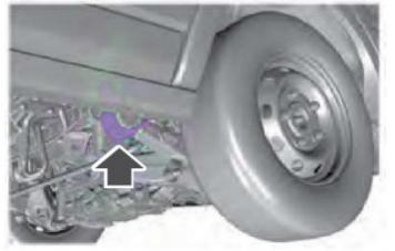
Position the head of the vehicle jack on the bolted body brackets.
