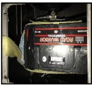
Place large looped strap around battery and tighten down
