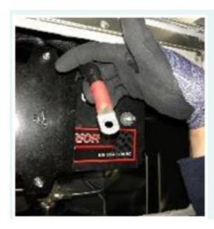
After removing nuts keep control of cables
