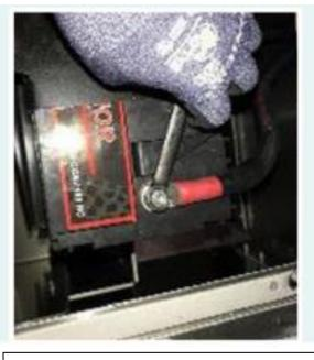
Using 9/16<sup>th</sup> wrench remove nuts from Battery terminals
