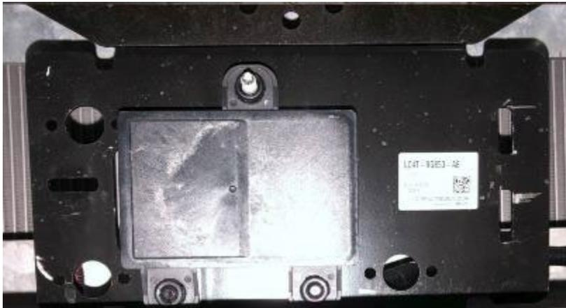
Fig. 1. Front of radar module and bracket assembly with cover removed
