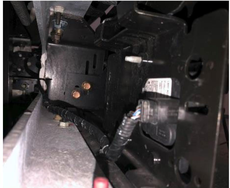
Fig. 2. Back of radar module and bracket assembly
