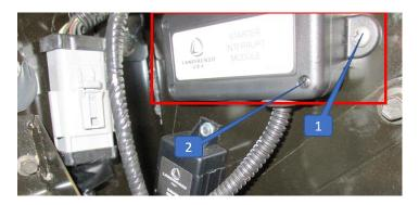
2. Once the relay is exposed unplug the connectors from the relay.
