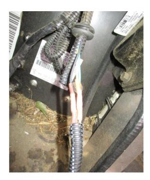
4. Lastly mount the new relay to the forward mounting hole by reusing one of the removed screws from step 1 (1) and tie up wires preventing rubs and chaffing.
