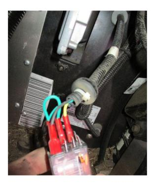
3. Using the new kit as a guide cut the 3 wires to length and then terminate by matching the colors together and using the provded heat shrink connectors
