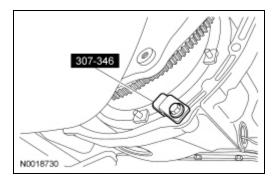
6. Align the index-mark made during removal.
