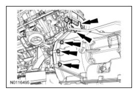
20. Slide the transmission back enough to install the Torque Converter Retainer and remove the transmission.
