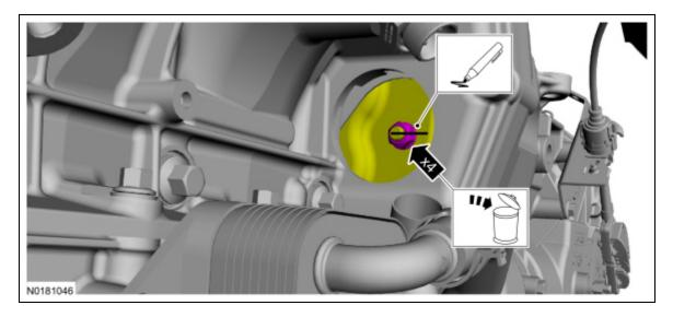
10. Remove the 2 bolts and the inspection cover.
