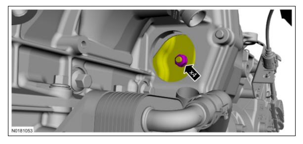
21. Install the torque converter access cover.
