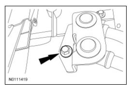
18. Remove the lower transmission fluid filler tube bolt and position the transmission fluid filler tube aside. Remove and discard the transmission fluid filler tube O-ring.
