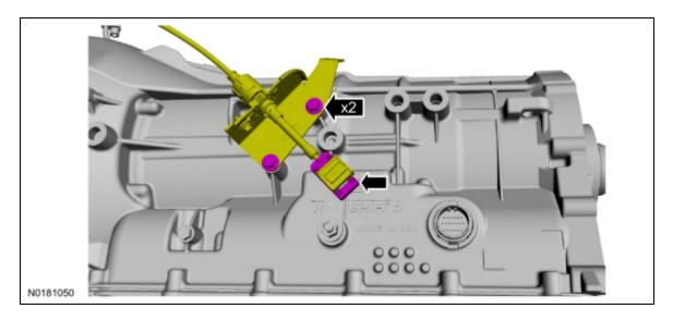
13. Remove the wiring harness retainers from the transmission case and position the wiring harness aside.
