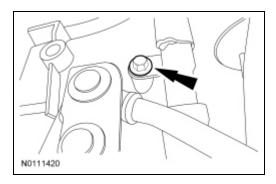
19. **NOTE:** Note the location of the 2 longer bolts for installation. The 2 longer bolts go to the bolt holes with the dowel pins.
