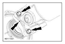
16. If installing a new, remanufactured or overhauled transmission, remove and discard the 4 transmission support insulator bracket bolts and remove the transmission support insulator and bracket.
