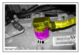
12. Disconnect the selector lever cable end from the manual control lever, remove the bolts and position the selector lever cable and bracket aside.
