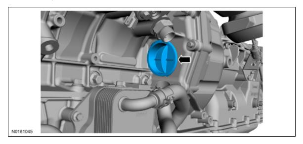
9. **NOTE:** Only rotate the crankshaft in a clockwise direction.
