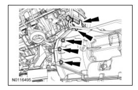
8. Install a new transmission fluid filler tube O-ring. Lubricate it with clean transmission fluid.
