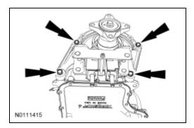
17. Remove the bolt and position the transmission fluid cooler tubes aside.
