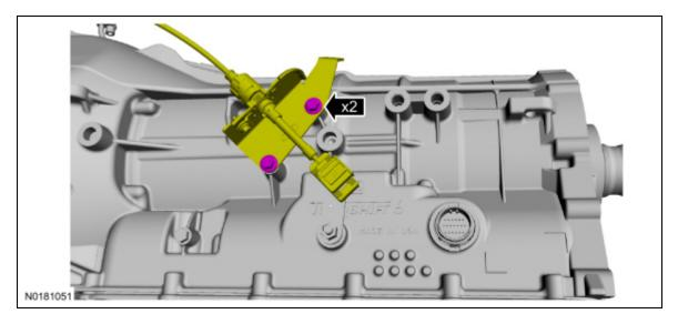
18. Install the transmission vehicle harness connector and lock the transmission vehicle harness connector by rotating the outer shell clockwise.
