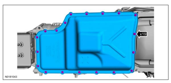
7. NOTE: The transmission fluid pan gasket is a reusable gasket.
