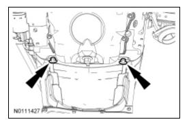
11. Rotate the shell of the transmission vehicle harness connector counterclockwise and disconnect the transmission vehicle harness connector.
