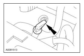
3. Remove the transmission fluid fill tube nut.
