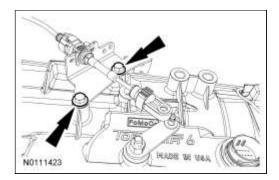
17. Install the transmission vehicle harness connector and lock the transmission vehicle harness connector by rotating the outer shell clockwise.
