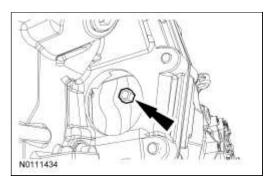
20. Install the torque converter access cover.
