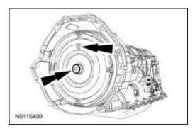
**NOTE**: Be sure to position the Torque Converter Retainer in the proper position to ensure the torque converter is held securely in place.
