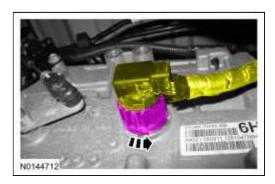
11. Disconnect the selector lever cable end from the manual control lever, remove the 2 bolts and position the selector lever cable and bracket aside.
