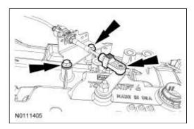
12. Remove the wiring harness retainers from the transmission case and position the wiring harness
