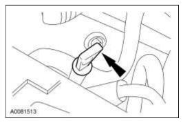
3. Remove the front transmission fluid fill tube bolt.
