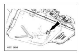
7. Remove the torque converter nut access cover.
