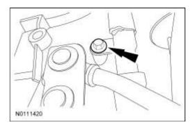
18. **NOTE**: Note the location of the 2 longer bolts for installation. The 2 longer bolts go to the bolt holes with the dowel pins.
