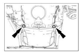
10. Rotate the shell of the transmission vehicle harness connector counterclockwise and disconnect the transmission vehicle harness connector.
