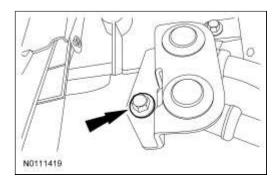
17. Remove the lower transmission fluid filler tube bolt and position the transmission fluid filler tube aside. Remove and discard the transmission fluid filler tube O-ring.
