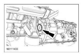
8. Remove and discard the 4 torque converter nuts.
