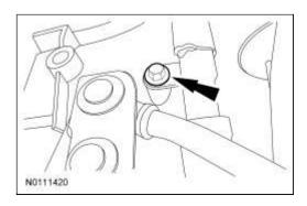
9. Inspect the transmission fluid cooler tube O-rings for damage and install new O-rings as necessary. Lubricate the O-rings with clean transmission fluid.
