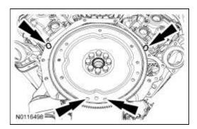
4. NOTICE: Prior to installation of the transmission, lubricate the torque converter pilot hub or damage to the torque converter or the engine crankshaft can occur.
