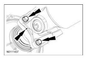
15. If installing a new, remanufactured or overhauled transmission, remove and discard the 4 transmission support insulator bracket bolts and remove the transmission support insulator and bracket.
