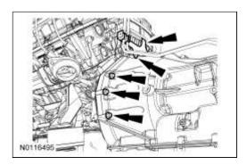
19. Slide the transmission back enough to install the Torque Converter Retainer and remove the transmission.
