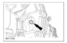
9. Remove the 2 bolts and the inspection cover.
