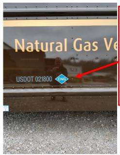
In the Horizontal: Centered between DOT decal and rivet.
