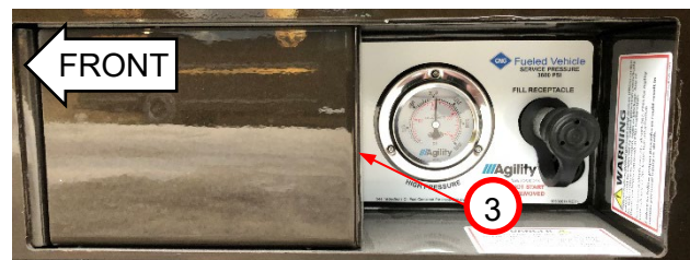
Figure 3: Fill panel cover (3) limits access to defuel valve and bleed valve.
