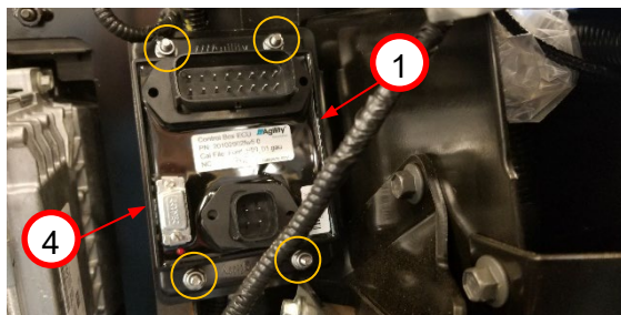
Figure 2: ECU (1), four corner ECU fasteners ( circled ), ECU bracket (4).
