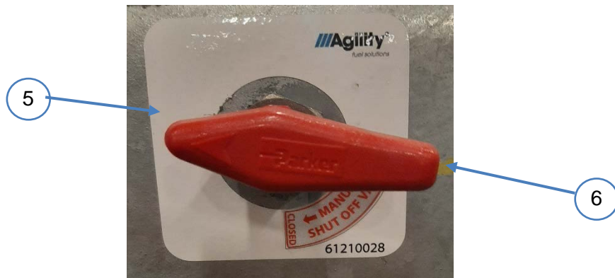
Figure 3. 1/4 turn manual shutoff valve (5) OPEN valve position (6)
