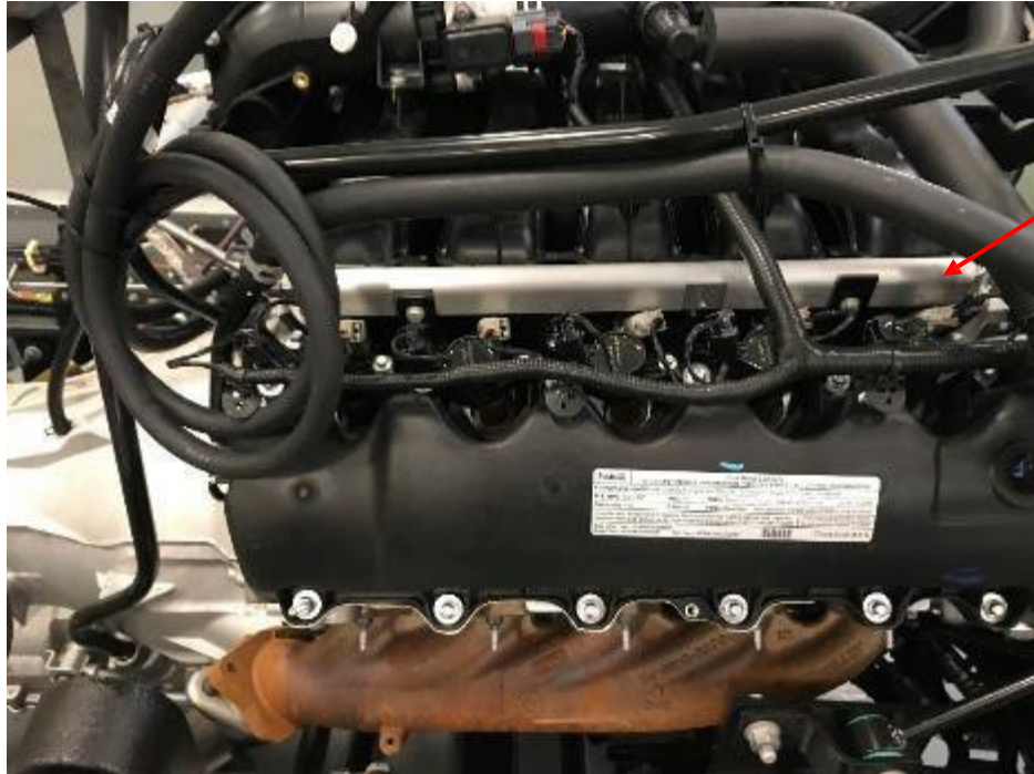
Fuel rail installed on passenger side of engine
