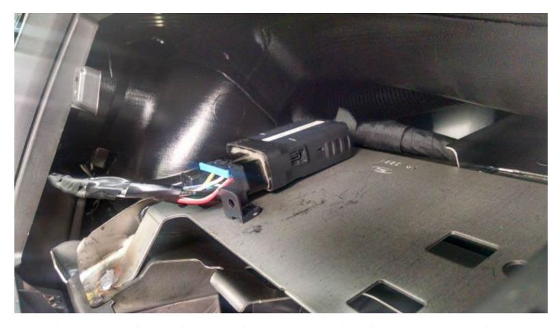
This picture shows the Geotab unit mounted in the connector and to the Instrument panel bracket. A piece of double sided adhesive tape can be used applied between the Instrument panel bracket and the Geotab unit if needed for possible rattle issues. The tape is not needed to secure the Geotab unit.
