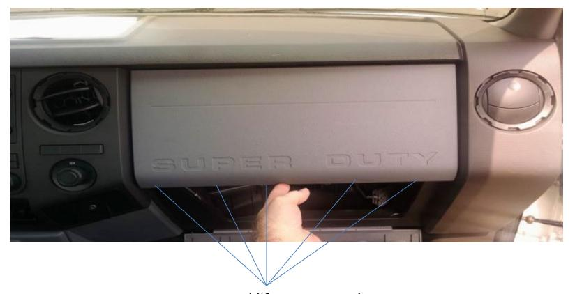
Remove 5 screws and lift out cover. The screws are 6mm hex head
