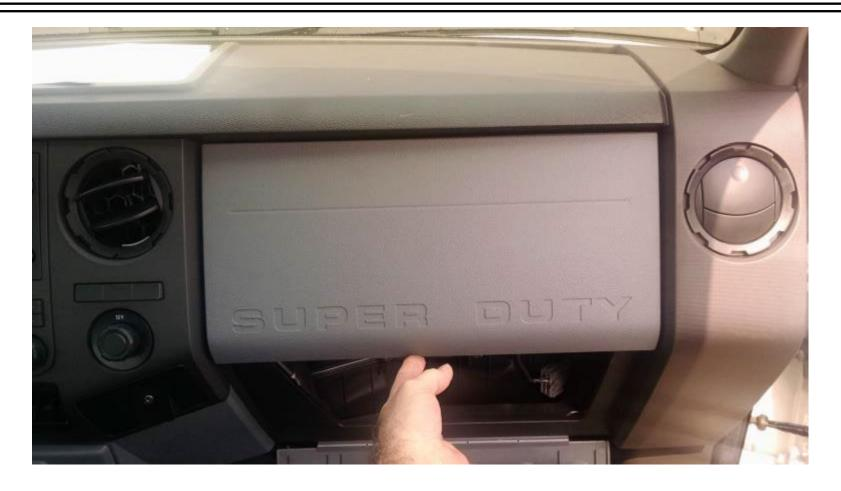
Re install the cover using the 5 screws. Raise the glove box door back into position
