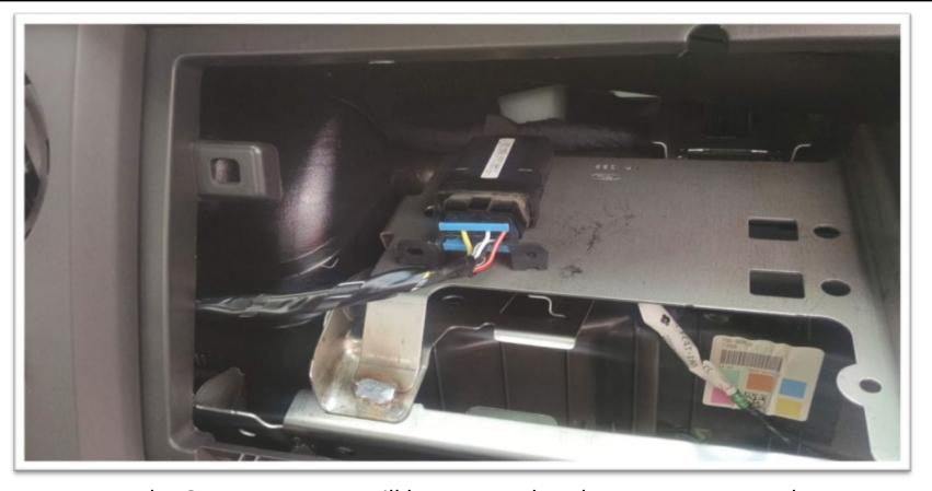
The OBDII connector will be mounted to the Instrument Panel bracket by the manufacturing plant. The customer or upfitter will connect the Geotab unit to the OBDII connector . The Geotab unit can only connect to the connector one way with the white label printed with the serial number pointing up.
