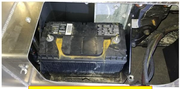
2. Remove vinyl wrap by sliding up. (it is not attached to tray or body).
