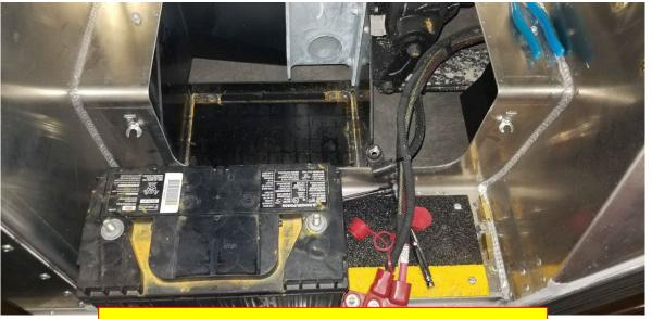
3. Slide battery forward, up and out.
