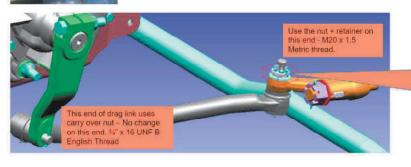
Torque, for latest Drag link only, is 250Nm (184 ft/lb) with the required hardware
