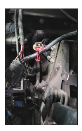
From Vicotr Edgell on 2/10/25: The harness that you are seeing with the blown fuse is actually a rework harness that is not standard. This is intended to separate the Keyless system from the keyed switch on the IP. I am unsure how many units have been upfit with this harness, I believe it was a field campaign
