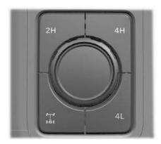
The drive mode control is on the instrument panel.
