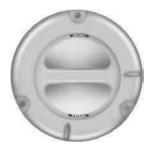
Your vehicle has manual hub locks on either the driver side or the driver and passenger side of your vehicle. For proper operation, make sure that each hub is fully engaged and that both hub locks are set to the same position (both set to lock or both set to auto). To engage lock, turn the hub locks completely clockwise. To engage auto, turn the hub locks completely counterclockwise.
