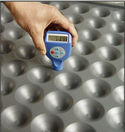
Panel Powder Coating Thickness Test
