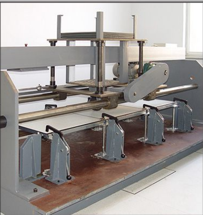
Rolling Load Test
