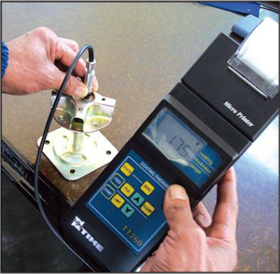
Pedestal Zinc Coating Thickness Test
