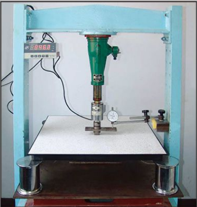
Concentrated Load Test
