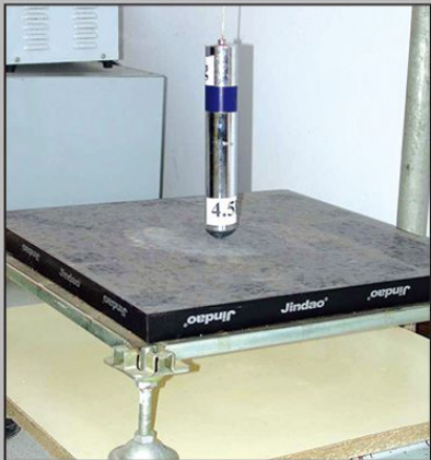
Impact Load Test
