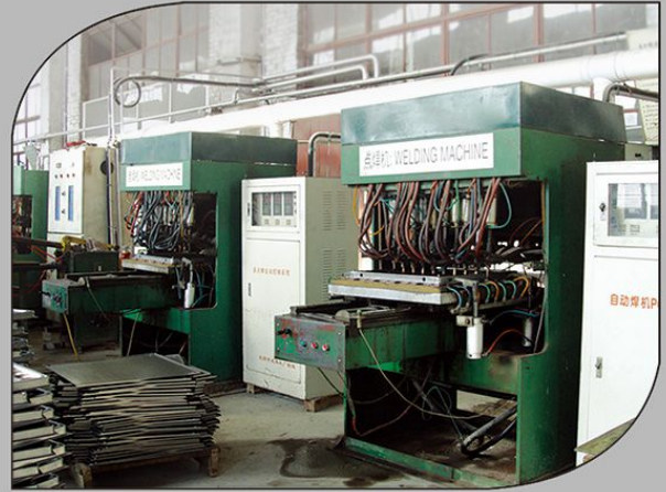
Automatic Welding Line
