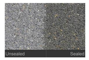
Applying a transparent concrete sealer to an exposed aggregate surface can improve both its performance and appearance. These sealers-typically film-forming acrylic resins-can help protect against spalling, dusting, efflorescence, freeze-thaw damage, stains, deicing salts, and abrasion. A sealer will also enhance the color of the aggregate, accentuating its depth and richness.
