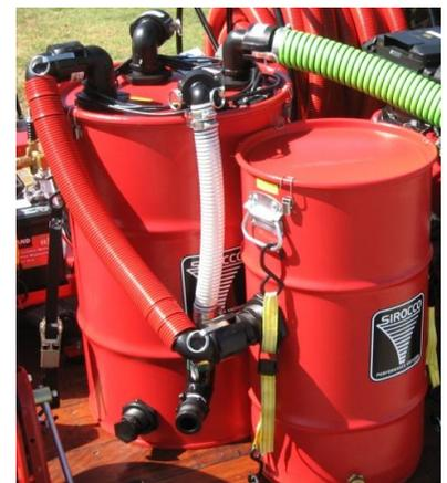
*Vacuuming Surface Cleaners-* The vacuuming surface cleaner is an important tool when cleaning sidewalks, driveways or parking lots, where runoff to storm drains must be avoided. They are also useful indoors, avoiding the extra step of mopping up the used wash-water. Attached to the vacuum system in place of, or in addition to, the VacuBerm, they provide a valuable time-saving, surface cleaning capability.
