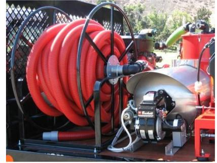
d) *Puddle Sucker*- A short version of the vacu-berm is the puddle sucker; its name gives away its purpose, draining puddles. This is an amazing attachment capable of sucking 25 Gallons of water per minute.
