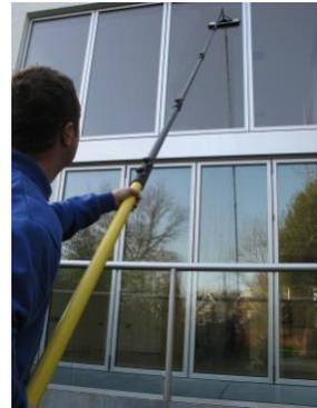
This process started to be used for window cleaning in the 1990s. **The process is the safest, most environmentally friendly, and fastest growing method used.** What happens is that by using pure water to rinse down glass, after agitation of the surface to loosen the dust and grit, this leaves the glass clean and "spot-free". There are two main ways of producing "pure water," reverse osmosis and deionization. Our equipment has taken this a step further and added a Carbon filter.
