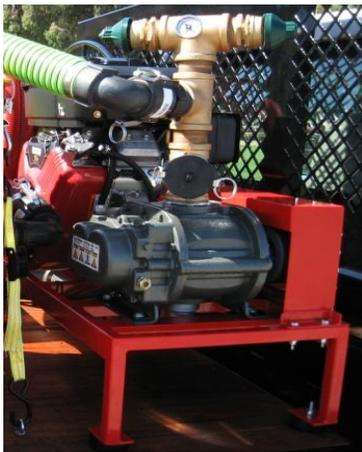
*Vacuum & Pump*- The heart of the wash-water recovery system is a powerful vacuum & pump. Our powerful unit consist of a 18 hp gasoline engine with belt drive to a positive-displacement blower style air mover, providing water lifts from 14 to 18 feet, and airflow rates at 650 cu.ft./min. This powerful unit allows multiple operators to use the system simultaneously.
