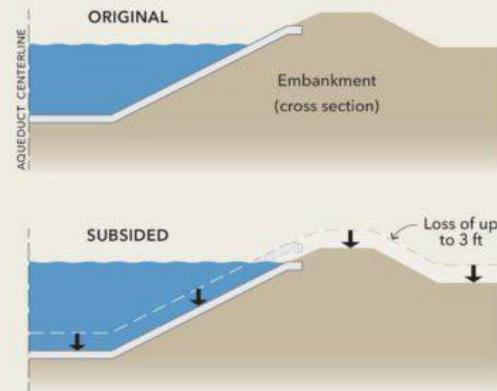
State Water Project operations decrease water levels to keep it below the (subsided) top of liner which means less flow capacity in the Aqueduct.
