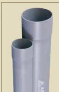
**SELFIT PIPES - (Type A & Type B) :** Selfit pipes are socketed on automatic socketing machine with self socket length (without groove). Such pipes are to be joined with solvent cement. One end of the pipe is plain and the other is self socketed on sophisticated automatic machines for high degree of accurate diameters. The pipes when joined using solvent cement, form a permanent water tight joint. **Sizes : 75 mm, 90 mm, 110 mm, 160 mm**
