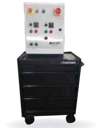
TOOL BOX MOUNTED OPERATOR CONTROL
