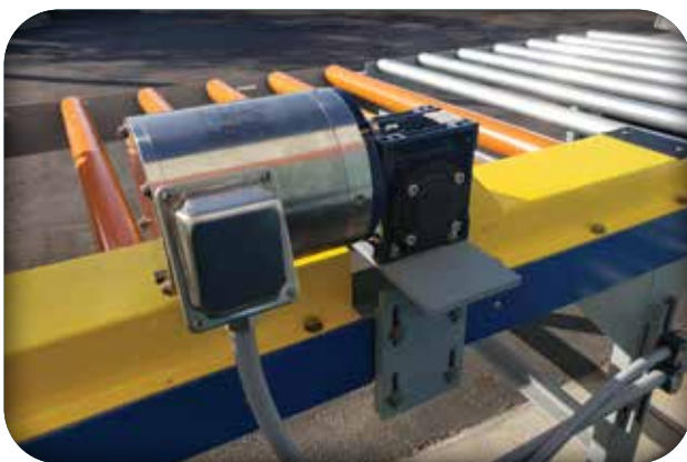
Stainless steel wash down rated motors
