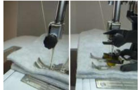
A dual feed foot can be used to match plaids perfectly. The photo below shows plaid fabric sewn together using Reverse Pattern Foot #1C. One fabric piece feeds slightly faster than the other causing the plaids to be mismatched. Plaids that almost match give the garment a “homemade” look.
