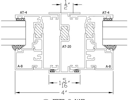
$\widehat{\text{14A}} \overset{\text{FIXED @ JAMB}}{\text{W/ STACK BAR}}$
