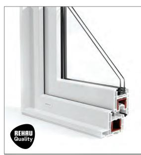
Performance summary Structural: up to CW-PG60 Acoustical: up to STC 43; OITC 34 Thermal: down to 0.17\* \* based on simulation
