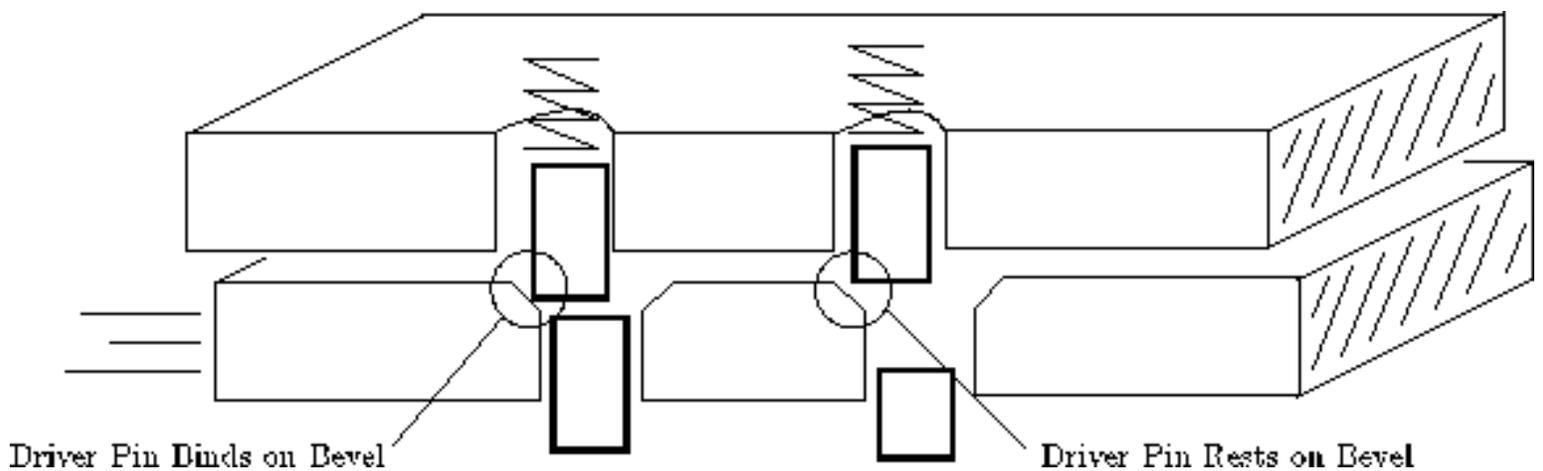
If you pick a lock and the plug stops turning after a few degrees and none of the pins can be pushed up and further, then you know that the lock has modified drivers. Basically, the lip of the driver has caught at the shear line. See the bottom of [Figure 9.7](#). Mushroom and spool drivers are often found in Russian locks, and locks that have several spacers for master keying.
