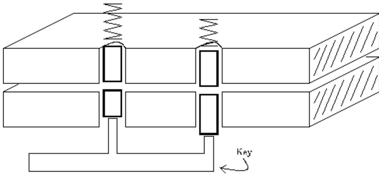
*Figure 3.3: (b) Proper key allows plates to slide*
