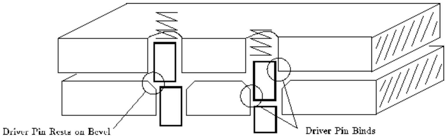
**Figure 9.6: (a) Driver jams on bevel**
