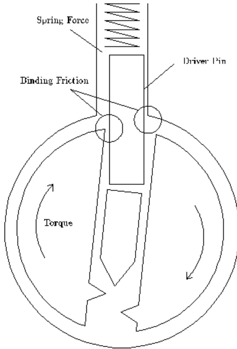
*Figure 5.3: Pins at the shear line*
