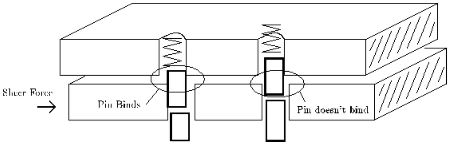
Figure 4.2: (b) Pick lifts the binding pin
