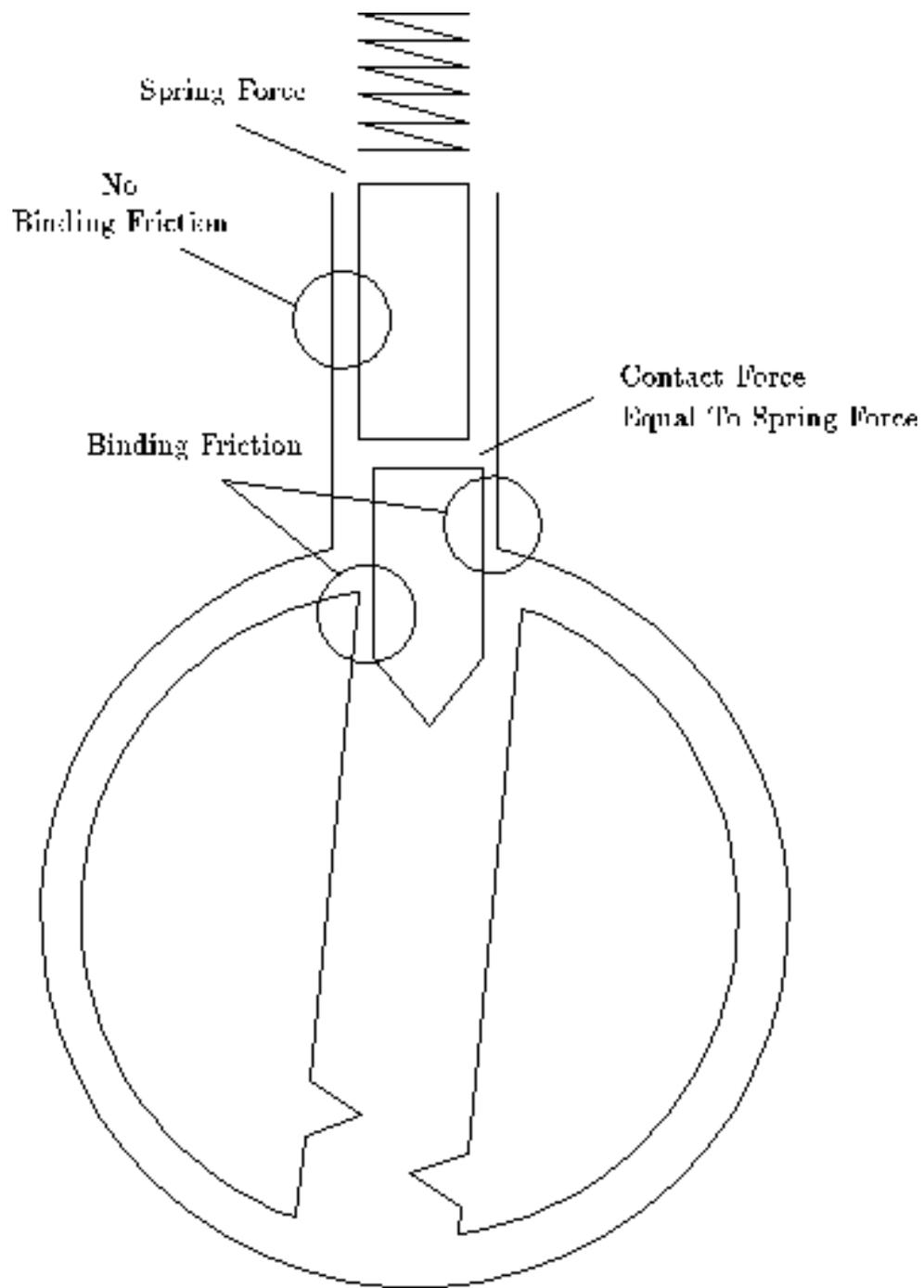
*Figure 5.5: Pressure required to move pins*
