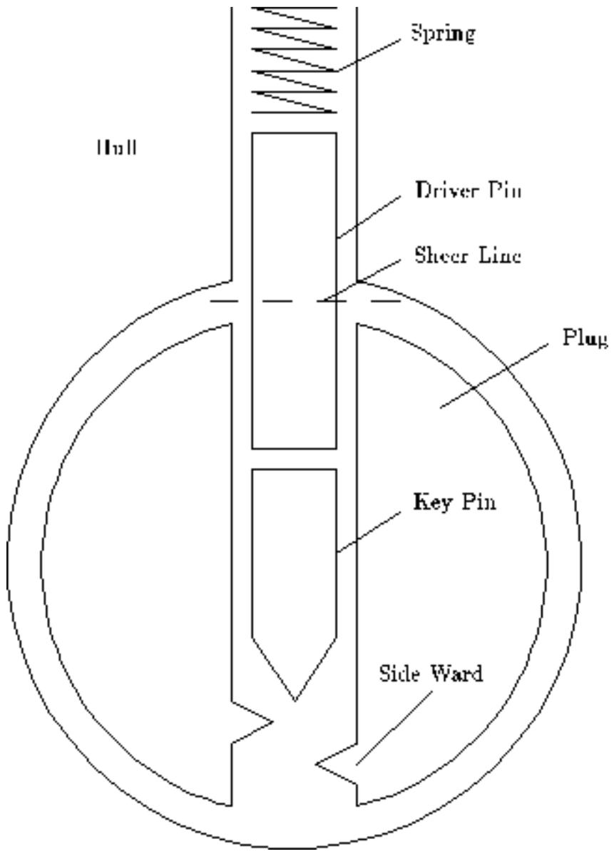
*Figure 5.2: Binding in the pin-column model*
