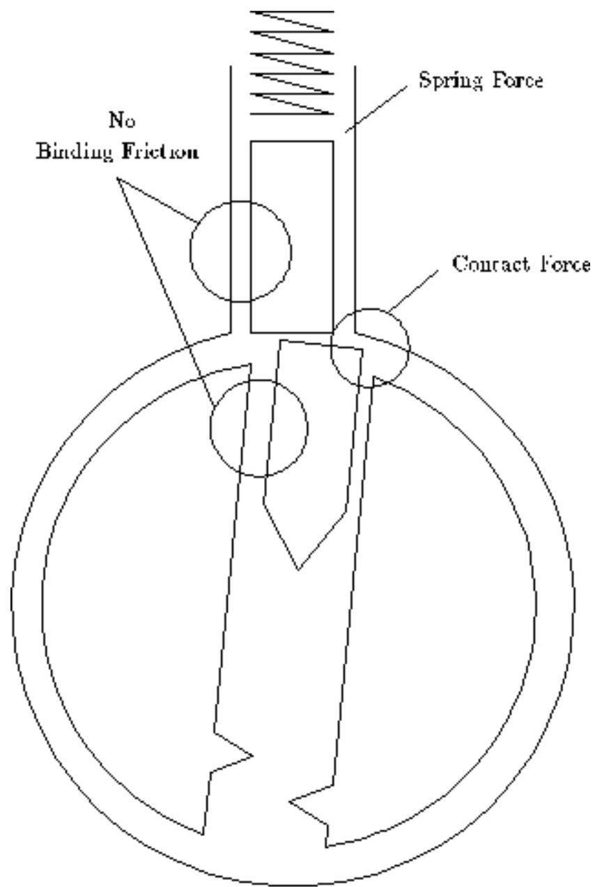
*Figure 5.4: Key pin enters hull*
