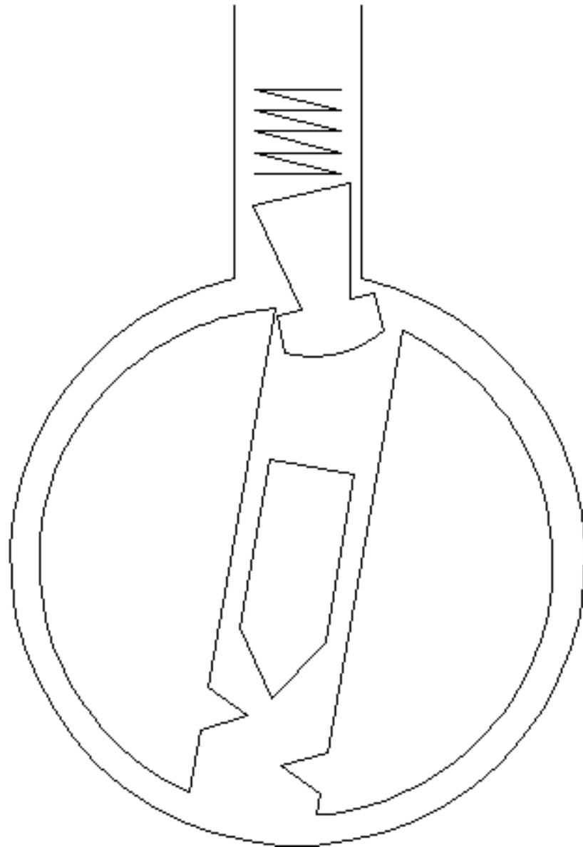
*Figure 9.8: Spacer pins for master keying*
