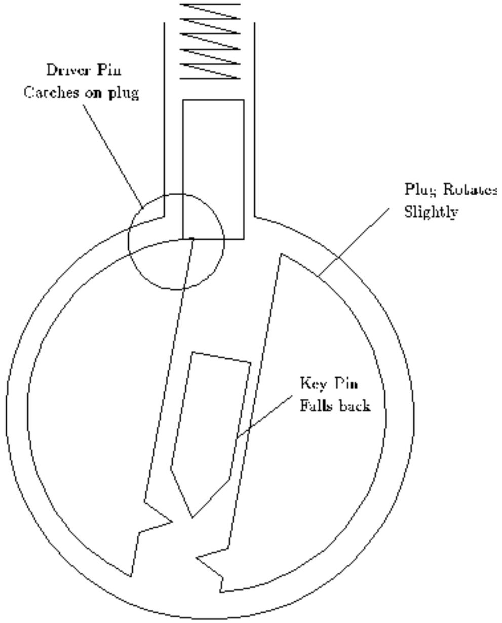
*Figure 6.2: Alignment of plug holes*
