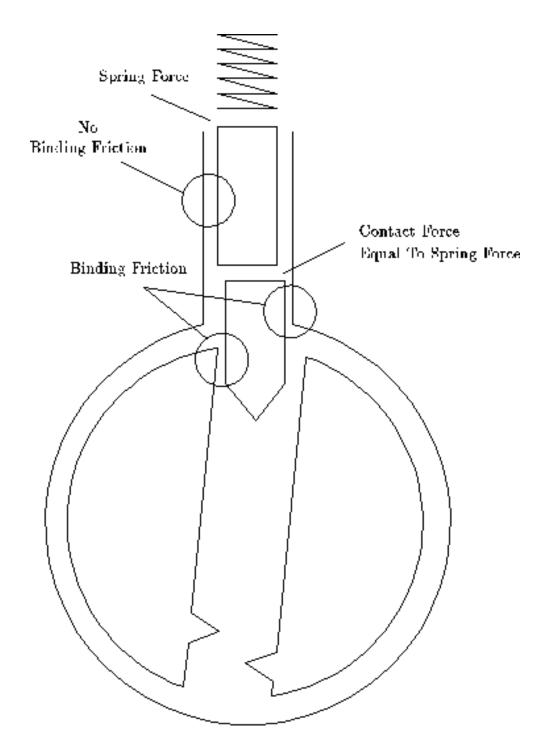
Figure 5.5: Pressure required to move pins
