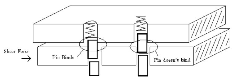
Figure 4.2: (b) Pick lifts the binding pin
