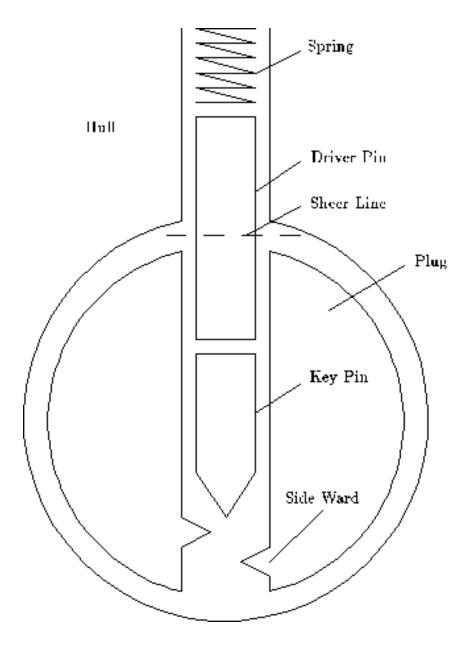
Figure 5.2: Binding in the pin-column model
