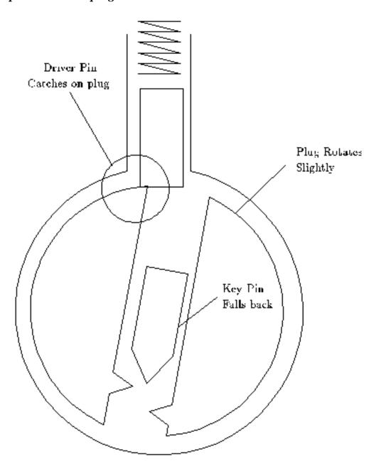
Figure 6.2: Alignment of plug holes
