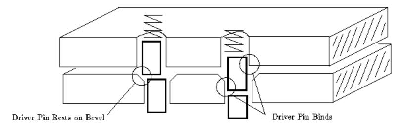
Figure 9.6: (a) Driver jams on bevel
