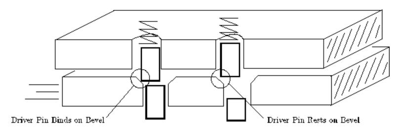
If you pick a lock and the plug stops turning after a few degrees and none of the pins can be pushed up and further, then you known that the lock has modified drivers. Basically, the lip of the driver has caught at the sheer line. See the bottom of <u>Figure 9.7</u>. Mushroom and spool drivers are often found in Russian locks, and locks that have several spacers for master keying.
