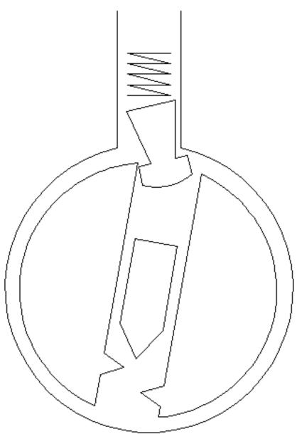
Figure 9.8: Spacer pins for master keying
