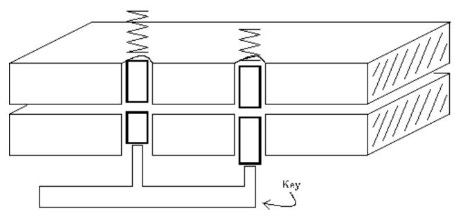
Figure 3.3: (b) Proper key allows plates to slide
