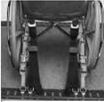
The Parallel Lap Belts attach directly to the floor track or plates, and provide an occupant restraint system that secures the passenger separately and independently from the mobility aid securement system.
