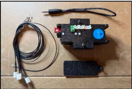
Fig. 1 (Left) - ESAD Components — clockwise from left - connectors, Safety #1 - Speaker Plug, ESAD top face with Safety #2 - Red Block, and battery door visible
