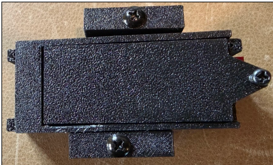
Fig. 9 - Battery door closed with screw closure on right
