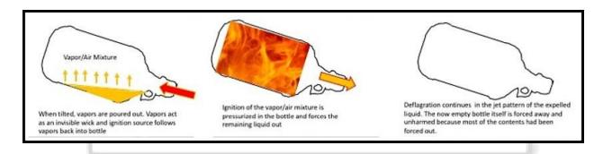
Flame Jetting occurs when a container, partially filled with a flammable liquid also holds gasses inside, and is poured on an open flame, ember, coal, etc.
