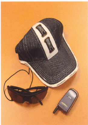
Covert Hat Camera, Cell Phone camera and Sun Glasses camera. All record to a remote Digital Video Recorder (DVR) with Date & Time stamp.
