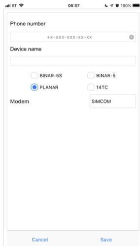
Enter the modem sim number and mark planar and make sure modem is set to simcom.
