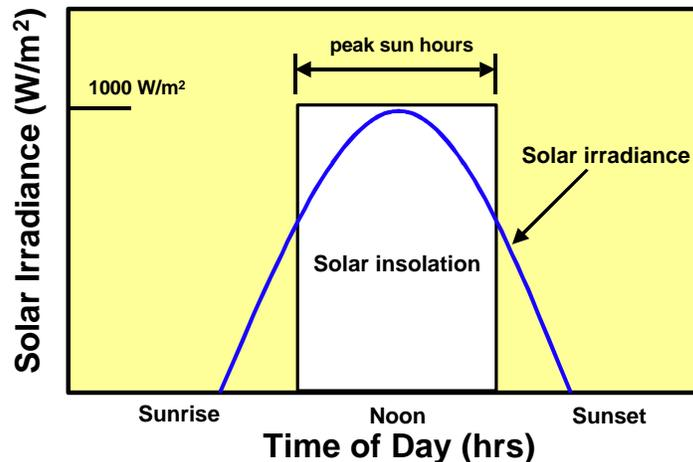
**Figure 9. Relationship between solar irradiance and insolation.**
