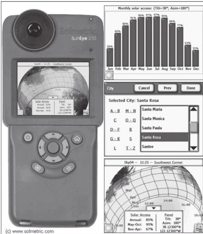
Figure 4.8 The Solmetric Suneye is a popular device used for shade analysis and can predict the path of the sun throughout the year.
