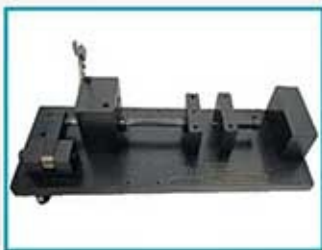
RELATION GAUGE WITH PUNCHING FIXTURE LEVER CHANGE SHAFT
