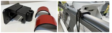
To mount the Scotty Side mount you can use 4 of a 10-24 x 1 inch screw with a 10-24 Nylock Nut works well to mount the scotty side mount. You should always try to use stainless screws. (Not Included)
