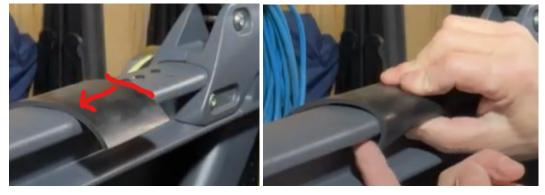
3. Insert each side of the Air Connects over the top of the adhesive rubber you just placed onto the rail. Inserting at a slight angle and then straightening them up to meet. Be sure they meet exactly or your screw holes will not line up.
