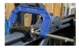
8. Place the lock nuts into their slots and begin to tighten the bolts, being careful not to cross thread, just get them both snug. Once they are snug you can begin to tighten the bolts.
