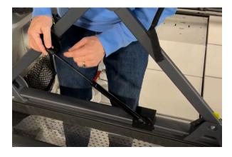
With the struts connected remove your arm supports, but be careful because the bimini can come down at this point. Lower the bimini to test the motion of the system. When testing the motion be sure to lower it very slowly and watch the strut as you go all the way down slowly.
