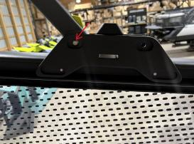
2. With the bolts removed insert the port (passenger side) lower mount into the slots as shown below. Please note: There are only two bolts not 3. You are not missing anything. We have an additional bolt hole in the location for a future accessory.
