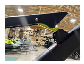
(13ft Compact Switch Lower measurement view. Measure from the lower weld 3  $\frac{1}{4}$  inches) and place a pencil mark/line where the edge of the gasket will line up with.
