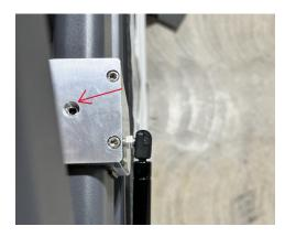
3. Next using a battery drill with a phillips head, screw in the set screws being careful not to overtighten the set screw or strip out your screw head. You will feel it stop.
