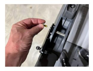
5. Now we can insert our ball stud bolt and nylock nut and tighten it down.
