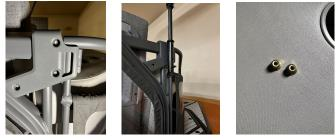
2. Using the new bolts included with the mount insert the new bolts through the bolt holes in the front and out the back of the mount. Then insert the mount with the bolts into the existing gate cover slots. Note: Insert the top bolt first and then using the lock nuts we saved from step get the nut started on the bolt. DO NOT TIGHTEN AT THIS POINT.
