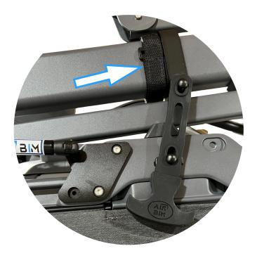
2. Next we will install the upper arm rail mount. Place one of the two gaskets close to the existing stock strap we just wrapped up keeping the gasket about ¼ inch or less away. The gasket should wrap around the arm meeting in the center of the arm. Please note the gasket and mount will be mounted facing forward to the front of the boat NOT behind the strap.
