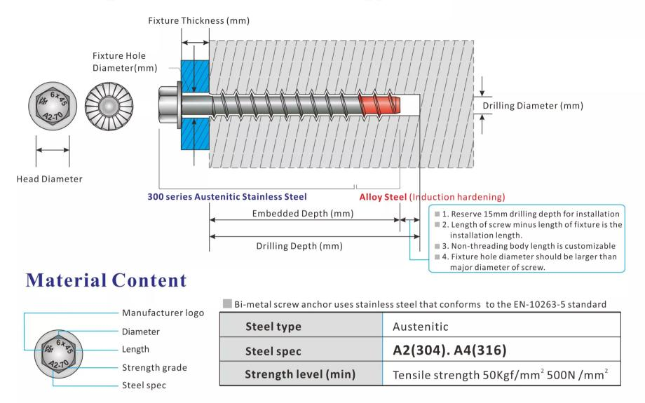
Threaded screw anchor comes with many distinguishing benefits such as their non-expanding, removable characteristics, among many others. The large diameter screw anchors and their nature to handle high loading jobs makes it natural for
