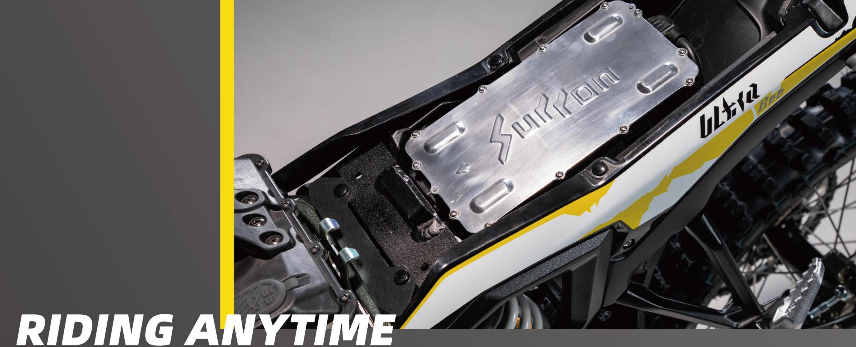
A hidden space under the seat is designed specifically for the Ultra Bee's charger.
