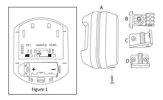
Remove back cover by unscrewing bottom screw and pull back cover from bottom to top. Install One (1) Panasonic CR123A, 3 VDC, 1550 mAh or equivalent lithium cylindrical battery Use only the recommended replacement batteries (see Specifications). Be sure to observe the polarity.
