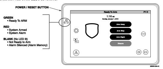
To reset the Touchscreen, press and hold the side **Power Button** for 3 seconds and then select the reset button  $\circlearrowleft$  on the screen to start the reset function. The Touchscreen can also be reset by pressing and holding the reset button for approximately15 seconds until the touchscreen resets automatically.
