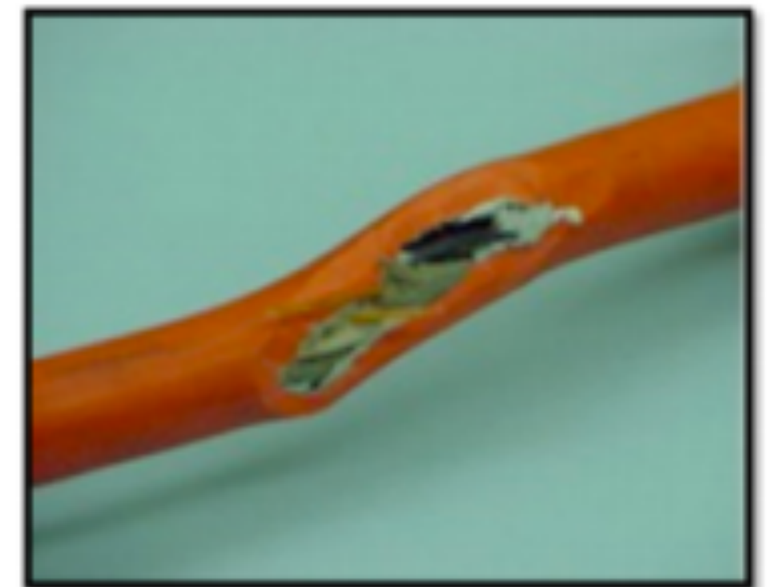
Image 2. Frayed Extension Cord
