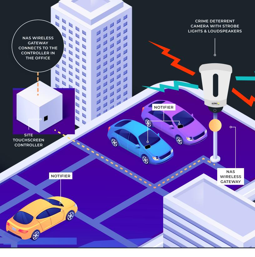
When a criminal individual tries to cut the exhaust, an alert is sent to the gateway with that vehicle's unique identifier for the controller to process, which then triggers the alarm and red/blue strobe lights on all the exterior Action-CS Active Deterrent Camera Units. The monitoring center then dispatches police or a security guard, even if they cannot see anyone. The agent can also talk down through the cameras to inform the perpetrator that police are on the way.
