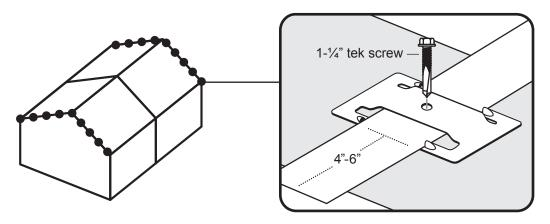
**1.3** Fasten these bands to the top flange of endwall rafters only, using a single 1-1/4" metal tek screw and banding clip. Pull banding hand-tight to far endwall rafter and secure in the same manner as above.
