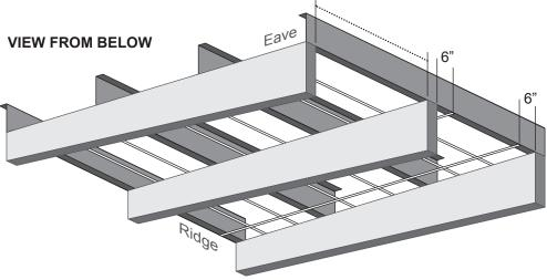
**2.1** Starting exactly six (6") inches from the rafter edge install a series of perpendicular (cross) bands to the bottom flange of the eave strut.
