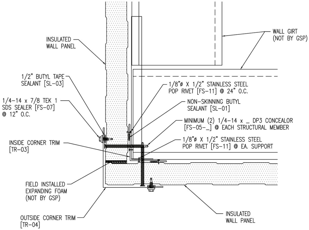
NOTE: FIELD CUT STARTING PANEL AND ENDING PANEL AS REQUIRED AT CORNER TRANSITION.
