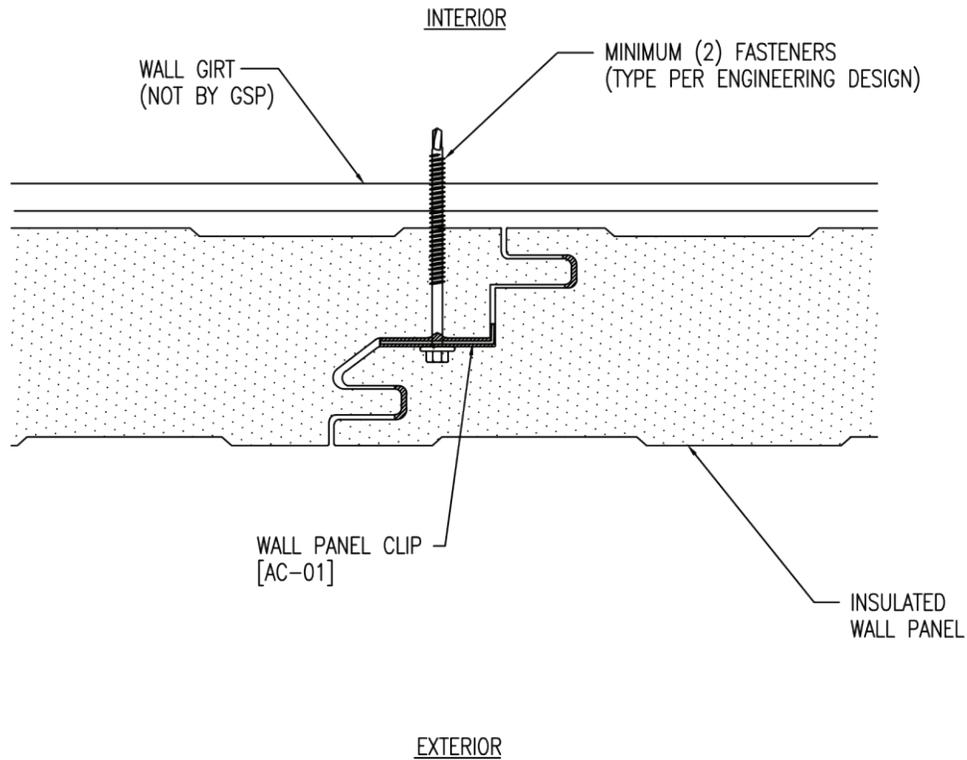
3/8" UNIFORM BEAD OF NON-SKINNING BUTYL SEALANT MUST BE APPLIED IN THE EXTERIOR FEMALE GROOVE. APPLYING SEALANT IN THE INTERIOR FEMALE GROOVE IS OPTIONAL DEPENDING ON VAPOR SEAL REQUIREMENTS
