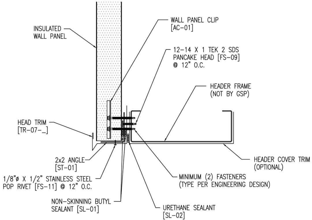
\*\* THE DETAIL SHOWN IS SUBJECT TO CHANGE WITHOUT NOTICE. PLEASE REFERENCE [WWW.GREENSPANPROFILES.COM](http://WWW.GREENSPANPROFILES.COM) FOR THE MOST CURRENT DATA \*\*
