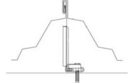
*"Triple Lok": A single mechanical seam process. -- "Quad Lok": A two-step mechanical seam process. This profile is typically used in high wind-load areas.
